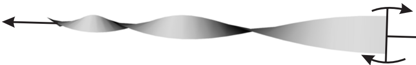
Fig. 7.7. A streamribbon demonstrates flow rotation by extruding a line along a streamline. Image credit: IRIS Explorer, synthetic data.
